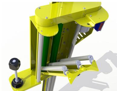
*The power pre-stretch carriage offers optimal load containment and minimal film usage. It also allows for easy film threading.*
