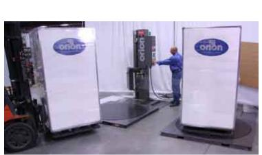
The carriage on the existing turntable easily reaches the second turntable.
